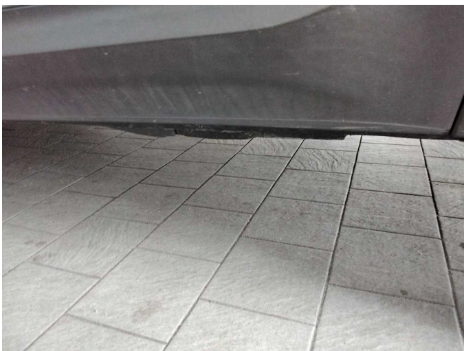
Damage 8: Door - rear left side: Brightware - lower - Scratch(es) - Smart repair
