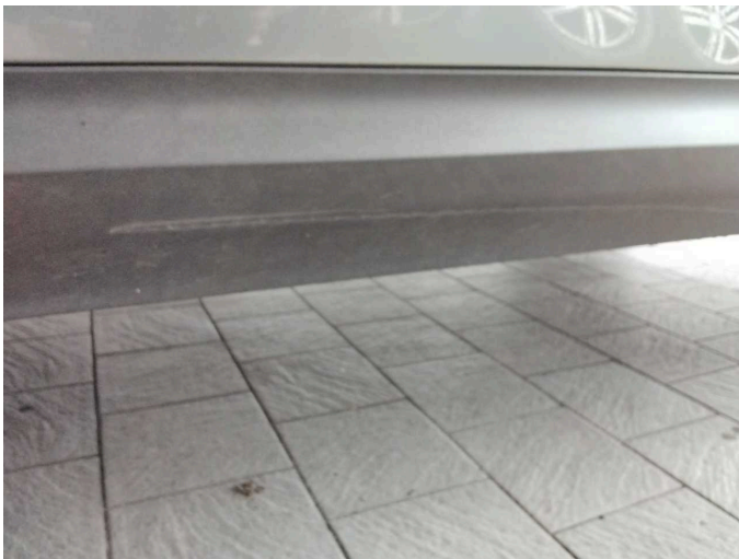
Damage 7: Door - front left side: Brightware - lower - Scratch(es) - Smart repair
