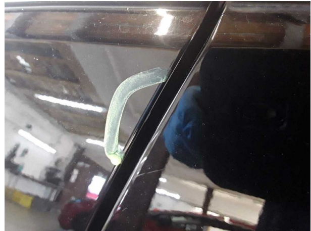
Damage #1: Door - front left side: Door edge - Scratched - Cover / polish
