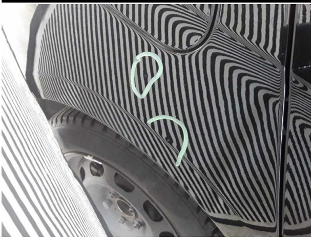
Damage #8: Side panel - rear right side: Side panel - Dent / paintcoat damage - Repair and paint
