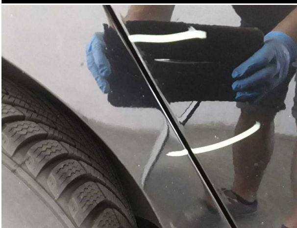
Damage #6: Door - rear right side: Door - Dent / paintcoat damage - Repair and paint
