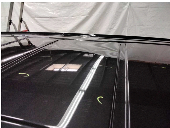
Damage 7: Roof: Roof - Damage by hail - Smooth repair work
