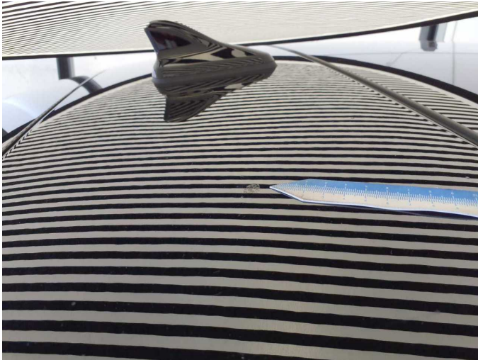
Damage 6: Roof: Roof (Anätzung) - Paint defect - Repair and paint
