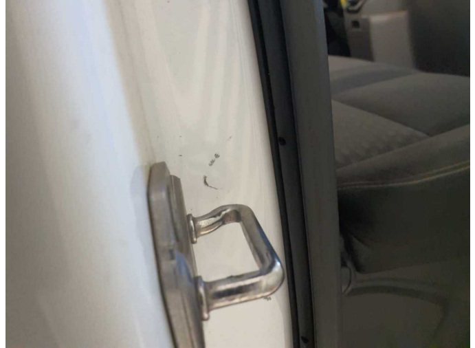
Damage 3: Body: B-pillar - right side - Dent / paintcoat damage - Smart repair
