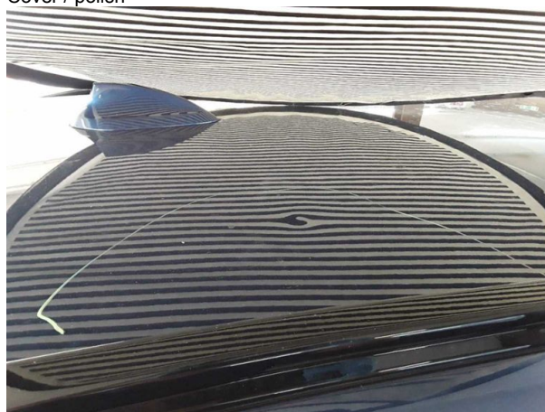
Damage #3: Roof: Roof - dent(s) - Smooth repair work
