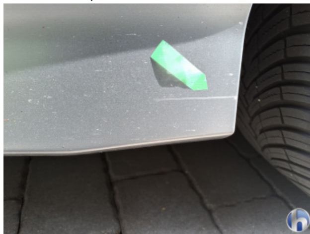
14. Schweller - Links Kratzer - Smart Repair
