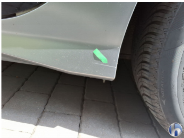
14. Schweller - Links Kratzer - Smart Repair
