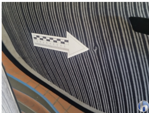
1. Tür Hinten - Links 1 Delle - Sanft Instandsetzen
