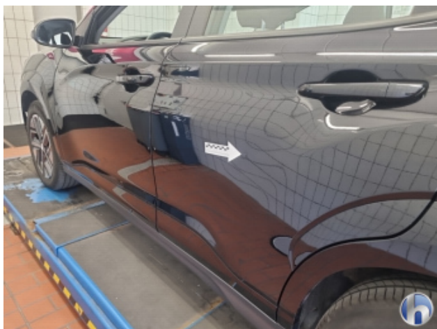
1. Tür Hinten - Links 1 Delle - Sanft Instandsetzen
