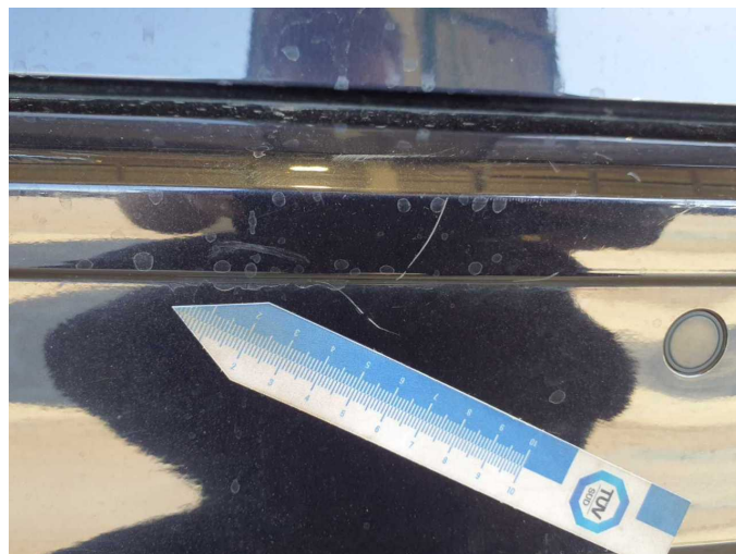
Damage 7: Rear bumper: Rear bumper - Scratch(es) - Paint
