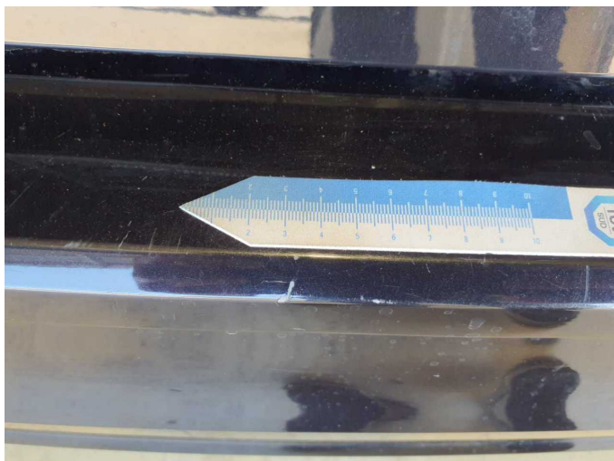
Damage 7: Rear bumper: Rear bumper - Scratch(es) - Paint
