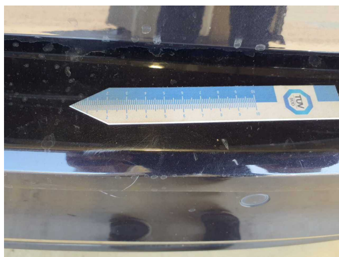
Damage 7: Rear bumper: Rear bumper - Scratch(es) - Paint
