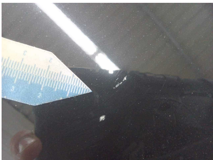
Damage 6: Bonnet: Bonnet - Stone chips - Paint
