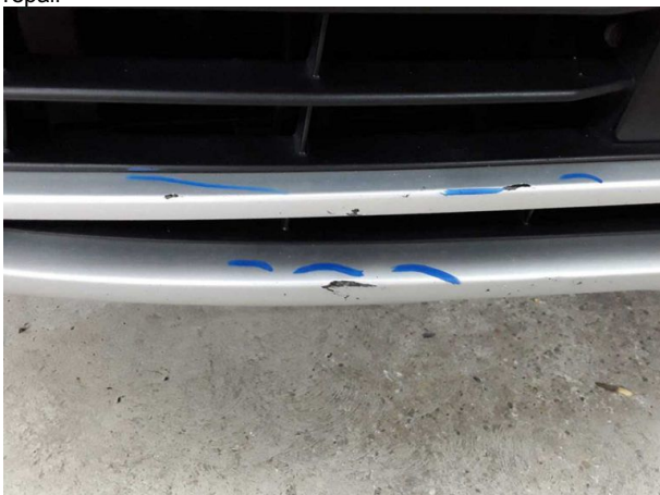
Damage #12: Front bumper: Spoiler - Scratched - Repair and paint
