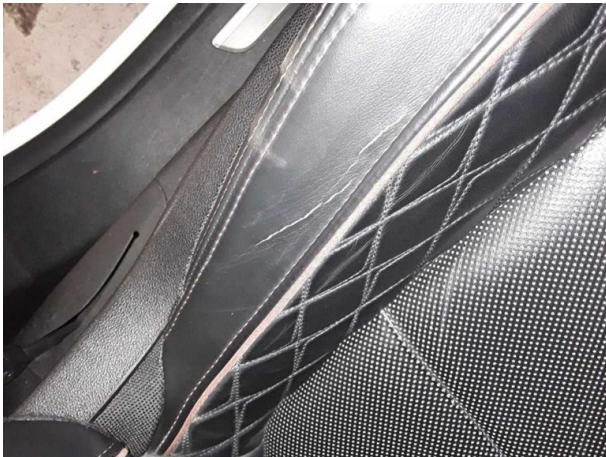
Damage #5: Seat - front: Seat cover - left side - Porous / cracked - Loss in value
