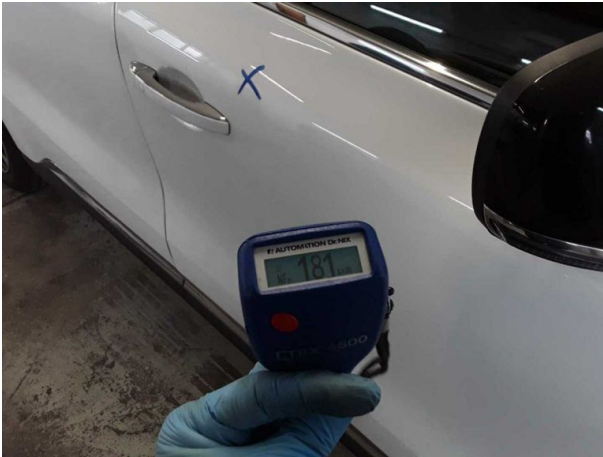
Repainting 1: Roof, Mudguard - right side, Door - front right side
