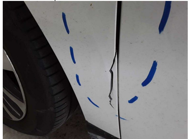
Damage #15: Mudguard - left side: Mudguard - left side - Broken / torn - Replace
