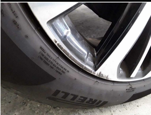
Damage #7: Wheel / tyres: Alloy rim - front left side - Scratched - Loss in value
