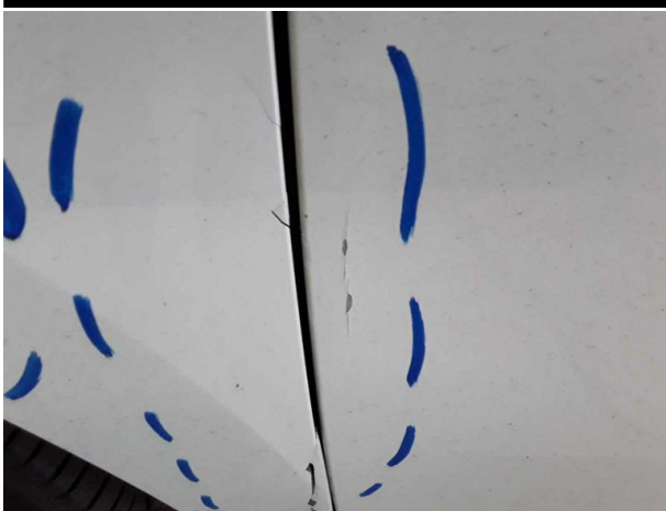
Damage #14: Door - front left side: Door - Dent / paintcoat damage - Repair and paint
