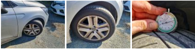
Tyre FL, Out of tolerance, Replace
