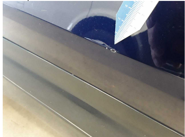
Damage #2: Door - rear right side: Door - Scratch(es) - Repair and paint
