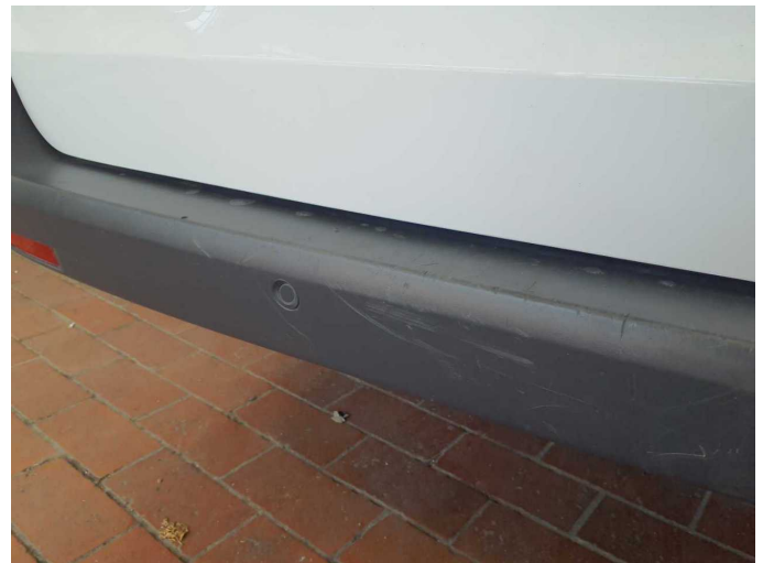
Damage 7: Rear bumper: Rear bumper - Scratched - Replace
