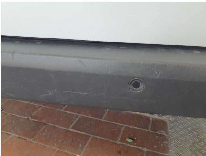
Damage 7: Rear bumper: Rear bumper - Scratched - Replace
