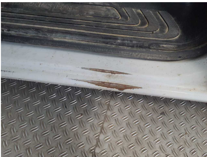
Damage 6: Sill - left side: Sill - Corrosion - Repair and paint
