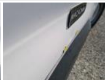
Side wall RR, Dent(s), Acceptable
