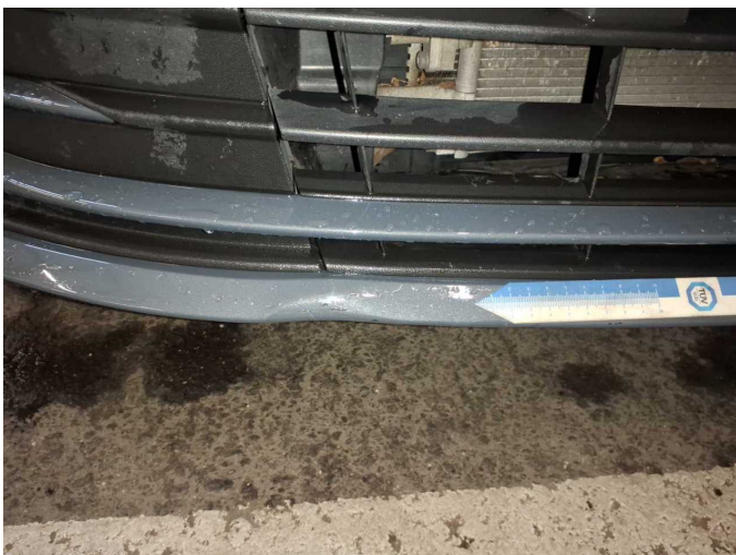
Damage 9: Front bumper: Front bumper - Deformed - Replace
