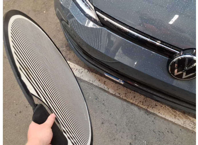
Damage 9: Front bumper: Front bumper - Deformed - Replace
