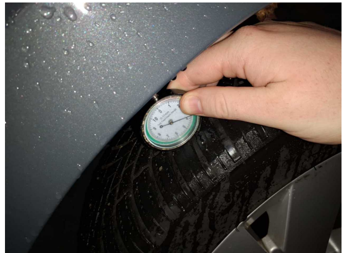
Damage 6: Wheel / tyres: Tyre - front right side - Does not meet the leasing specifications - Replace
