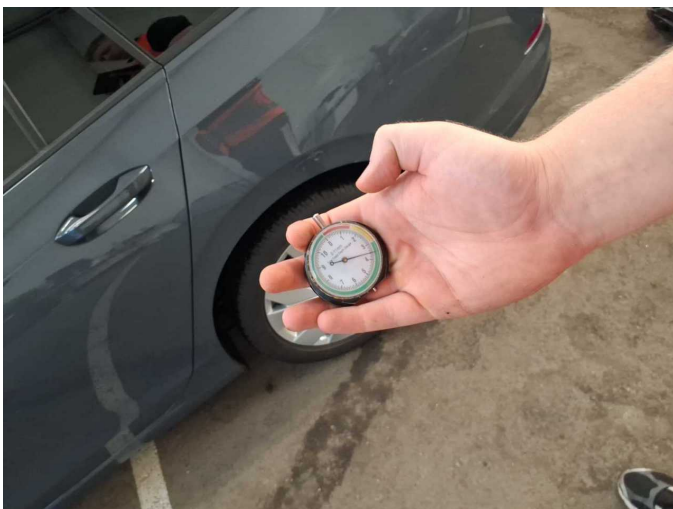
Damage 3: Wheel / tyres: Tyre - rear left side - Does not meet the leasing specifications - Replace
