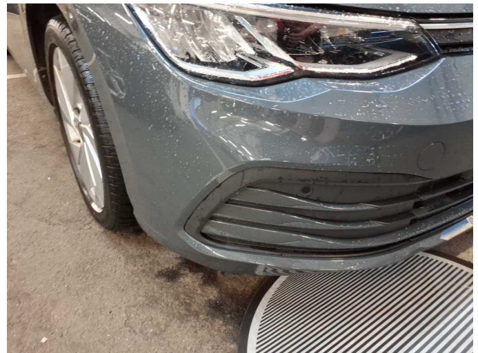
Damage 9: Front bumper: Front bumper - Deformed - Replace
