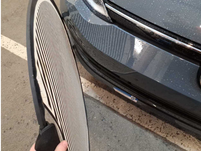
Damage 9: Front bumper: Front bumper - Deformed - Replace
