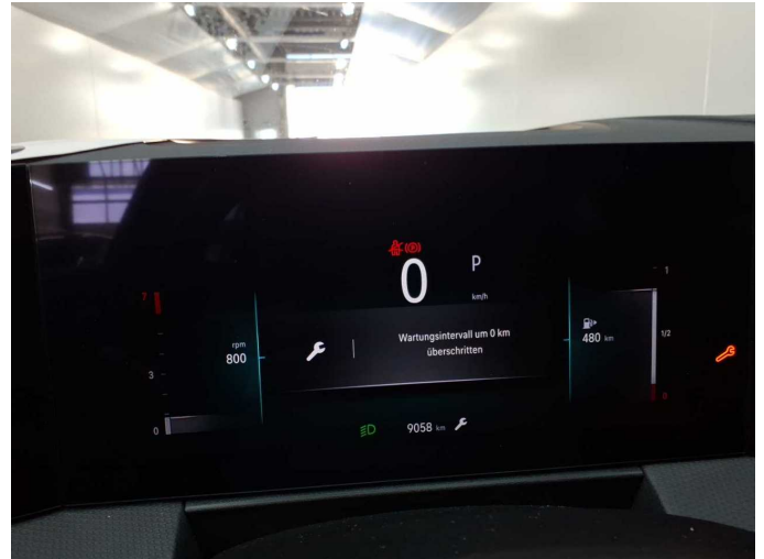
Damage 3: Misc.: Inspection / maintenance - Due - Replace
