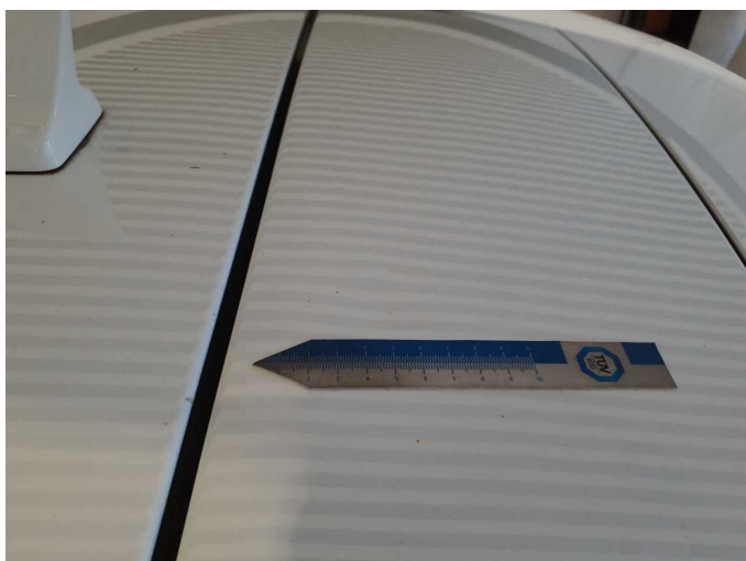
Damage 3: Boot lid / rear door: Rear spoiler - dent(s) - Smooth repair work
