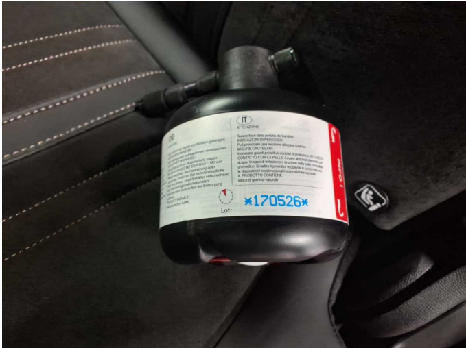
Damage 1: Equipment: Tirefit filler - Expired - Replace
