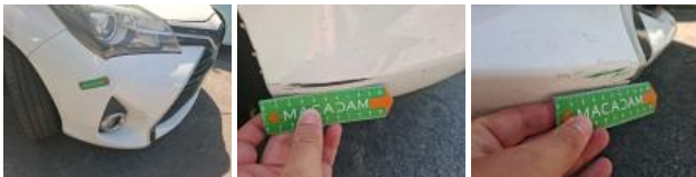
Bumper FR, Scratch(es), Repair and paint (complete)
