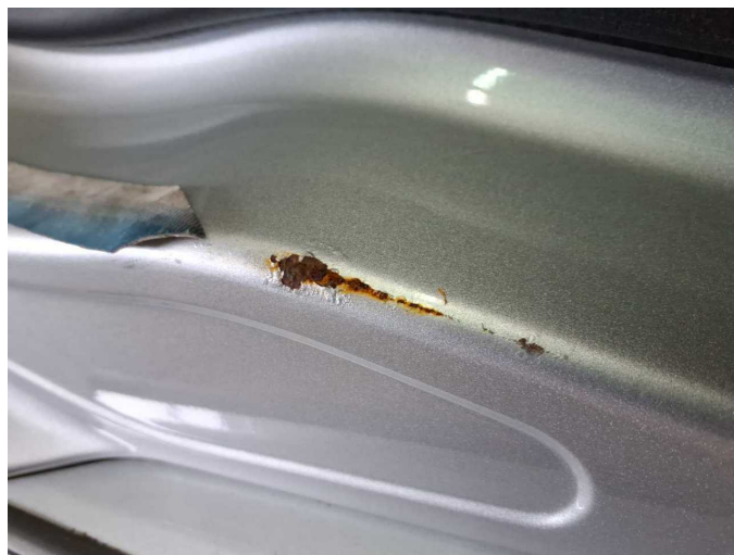
Damage 7: Side panel - rear right side: Sill - Corrosion - Paint
