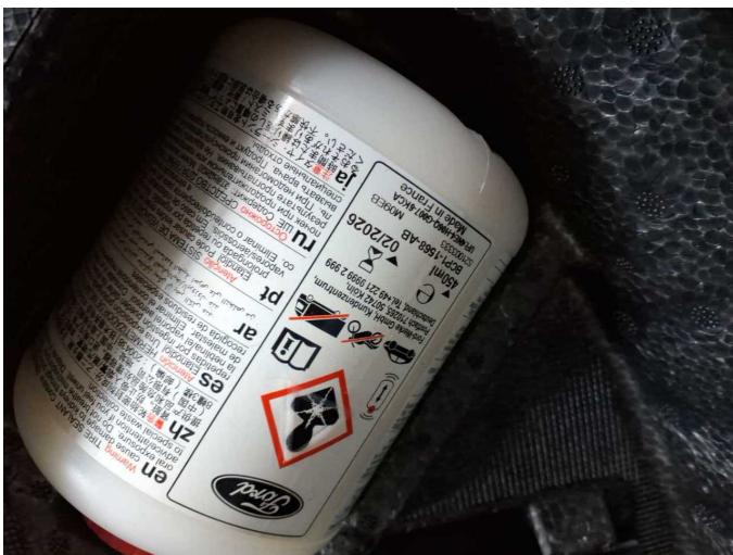
Damage 1: Equipment: Tirefit filler - Expired - Replace
