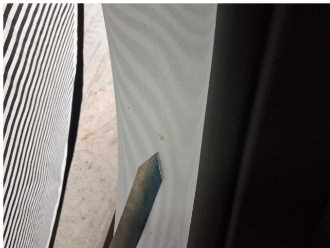
Damage 2: Body: B-pillar - right side - Dent / paintcoat damage - Smart repair
