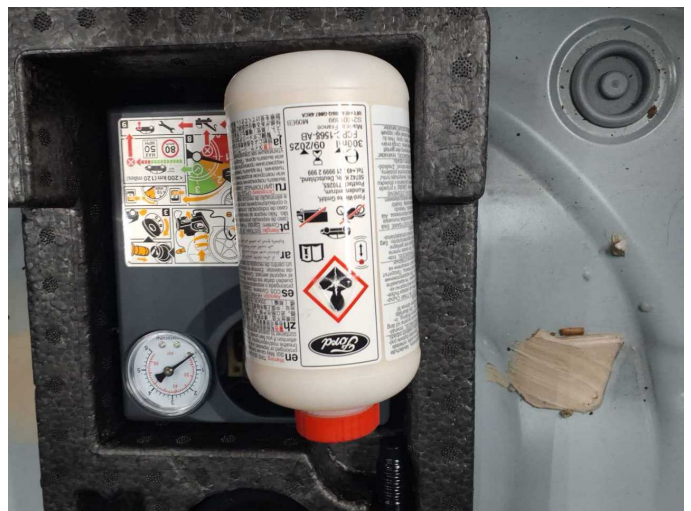
Damage 1: Equipment: Tirefit filler - Expired - Replace
