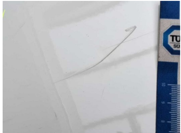
Damage #5: Bonnet: Bonnet - Scratch(es) - Repair and paint
