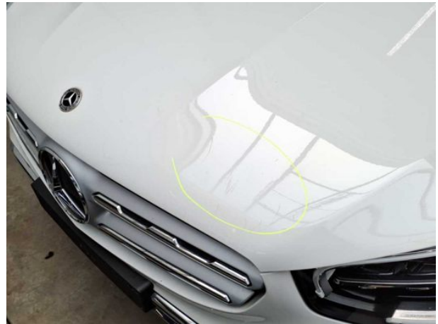
Damage #5: Bonnet: Bonnet - Scratch(es) - Repair and paint
