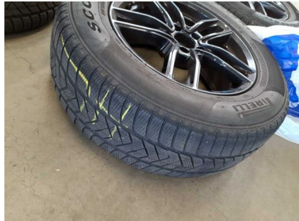
Damage #1: 2nd wheel set: 2 tyres (3mm im Fahrzeugliegend) - Worn - No deduction
