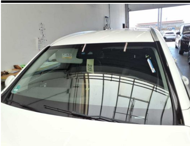
Damage #6: Vehicle glazing: Windscreen with lane departure assistant - Stone chips - Replace
