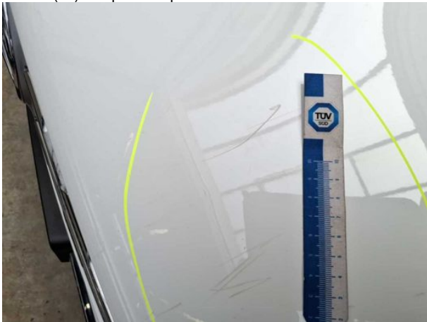
Damage #5: Bonnet: Bonnet - Scratch(es) - Repair and paint
