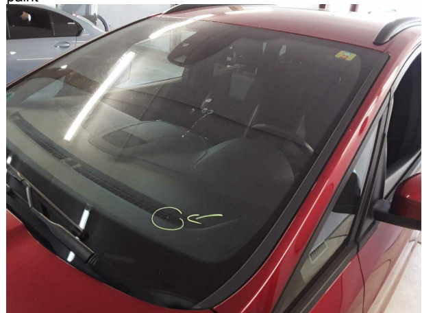
Damage #6: Vehicle glazing: Windscreen, heated (Rissbildun... - Stone chips - Replace
