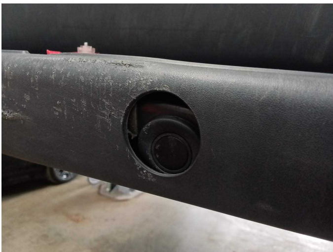
Damage 1: Rear bumper: Parking sensors - right side - Malposition - Replace
