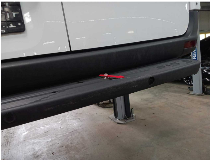
Damage 2: Rear of vehicle: Foot plate - Damaged - Replace
