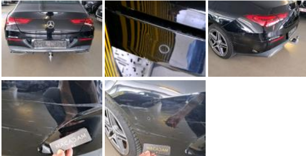
Alloy rim RR polished, Scratch(es), Repair and paint (complete)
