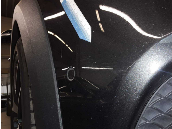
Damage 6: Front bumper: Front bumper - Scratched - Paint
