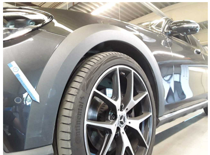
Damage 1: Mudguard - left side: Wheel well extension - Scratched - Loss in value
