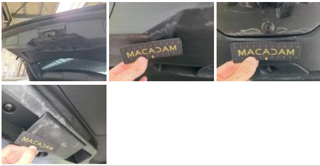
Bumper trim R, Scratch(es), Smart repair
