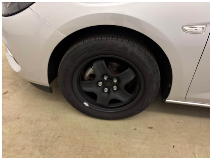
Missing part 1: Wheel / tyres: Wheelset - complete (Radkappen) - Missing - Replace
