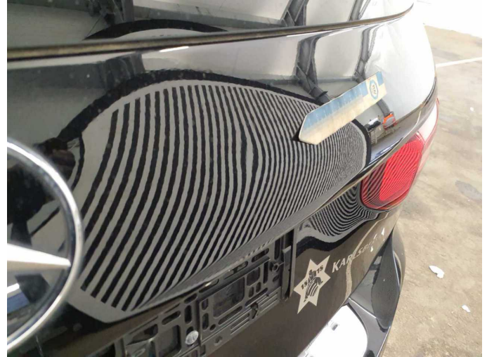
Damage 2: Boot lid / rear door: Boot lid - dent(s) - Smart repair
