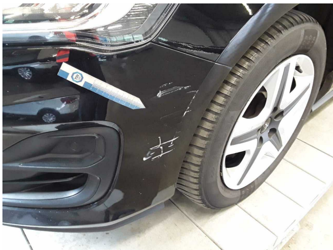
Damage 13: Front bumper: Front bumper - Scratched - Paint
