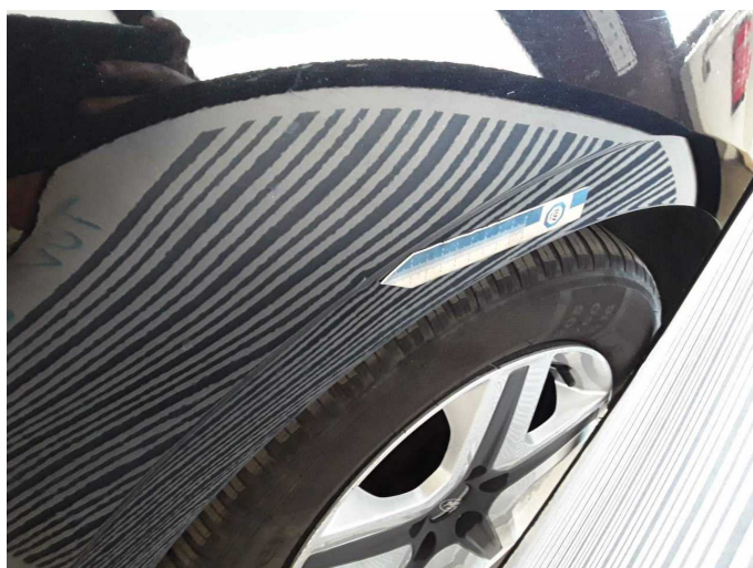
Damage 12: Mudguard - right side: Mudguard - right side (Delle auf Kante) - Dent / paintcoat damage - Repair and paint
