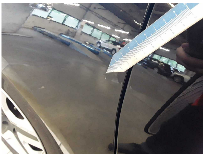
Damage 6: Mudguard - left side: Mudguard - left side - Scratch(es) - Smart repair
