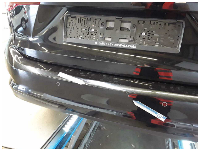
Damage 10: Rear bumper: Rear bumper - Scratch(es) - Paint
