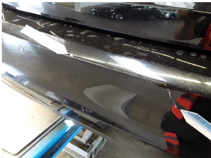
Damage 10: Rear bumper: Rear bumper - Scratch(es) - Paint
