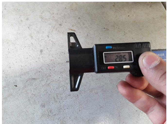
Damage 9: Wheel / tyres: Tyre - front - Worn - Replace
