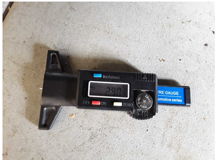
Damage 9: Wheel / tyres: Tyre - front - Worn - Replace
