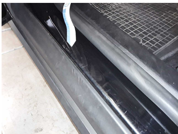
Damage 11: Sill - left side: Sill - Scratch(es) - Paint
