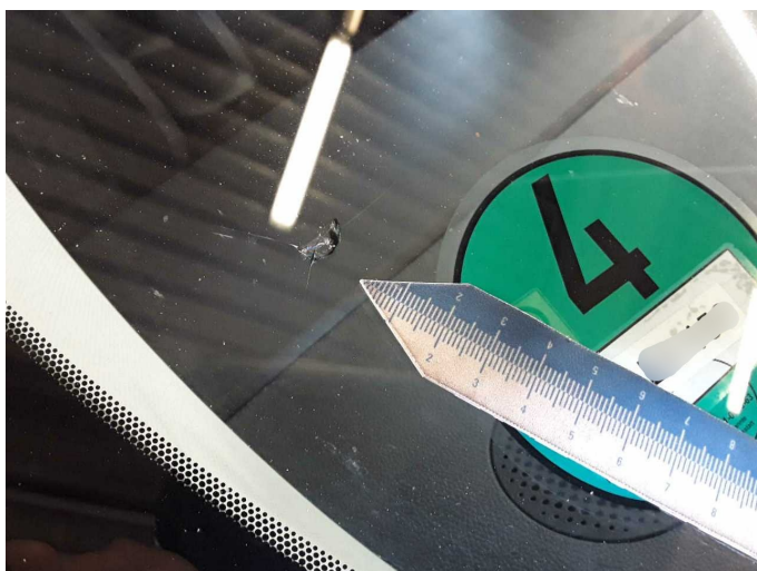
Damage 17: Vehicle glazing: Windscreen - Stone chips - Replace
