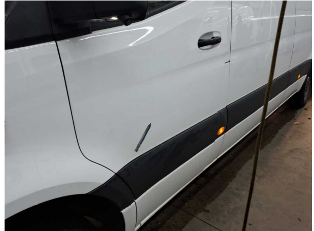
Beschädigung #9: Tür vorn links: Tür - Delle(n) - Smart Repair
