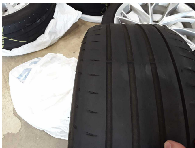
Damage 1: 2nd wheel set: 2 tyres - Worn - Replace
