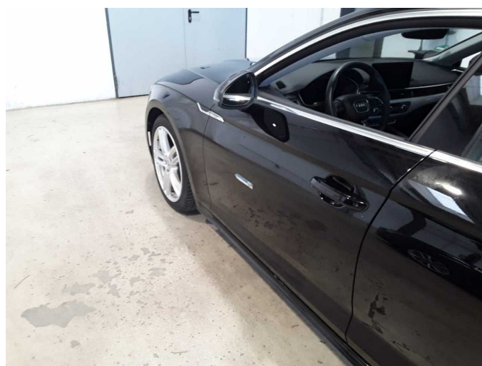
Damage 3: Door - front left side: Door - dent(s) - Repair and paint
