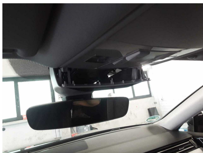
Damage 3: Instrument panel: Interior mirror - Damaged - Replace
