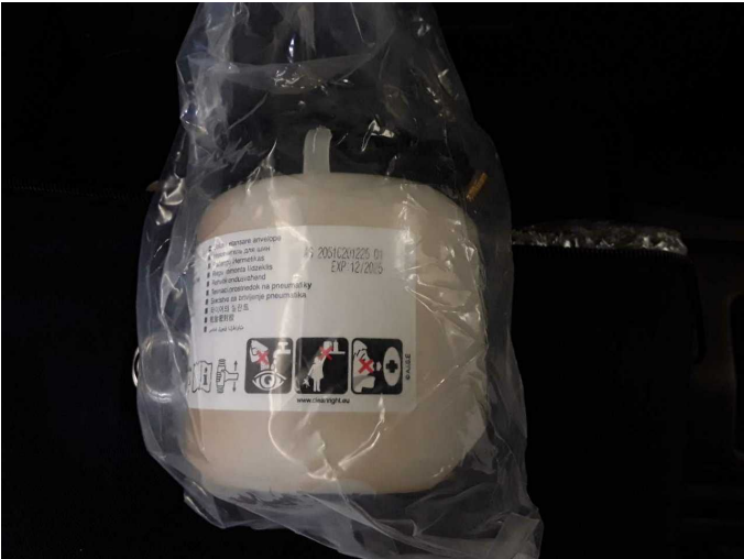
Damage 1: Equipment: Tirefit filler - Expired - Replace
