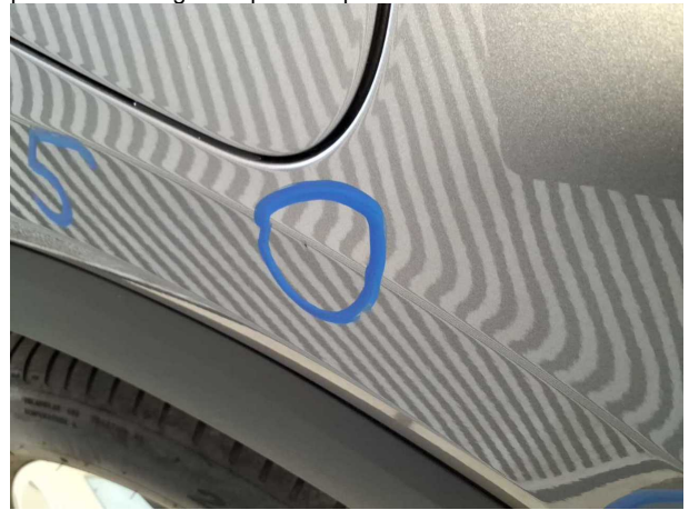
Damage #6: Side panel - rear right side: Side panel - Dent / paintcoat damage - Repair and paint
