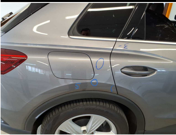
Damage #6: Side panel - rear right side: Side panel - Dent / paintcoat damage - Repair and paint
