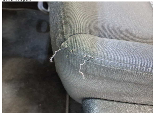
Damage #4: Seat - front: Seat cover - left side - Damaged - Replace
