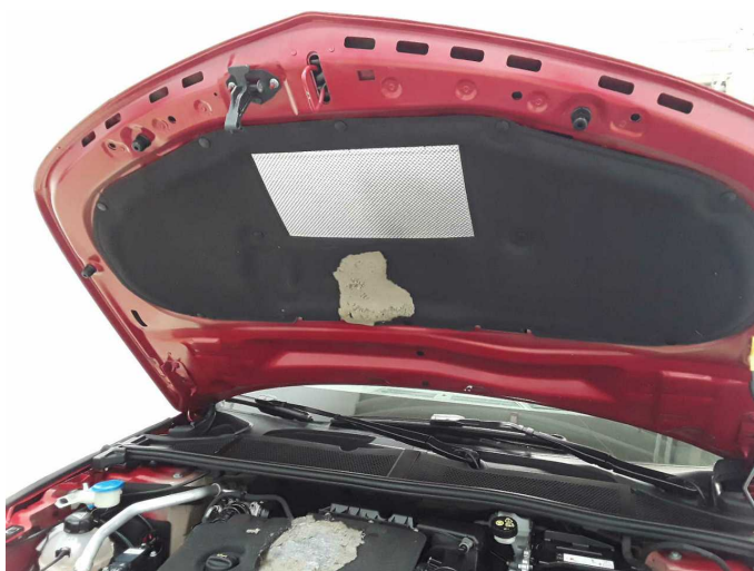
Damage 5: Bonnet: Insulation lining - Damage caused by marten / rodent - Replace
