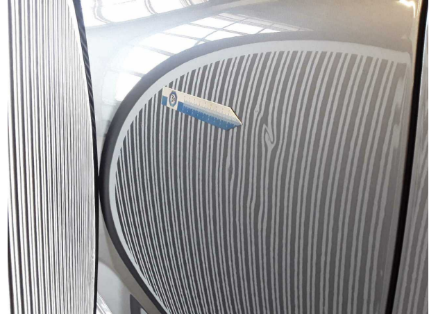
Damage #1: Door - rear right side: Door (4x) - dent(s) - Smoo... repair work
