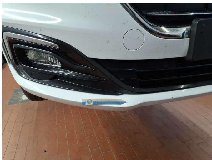
Damage 8: Front bumper: Front bumper - Deformed - Replace
