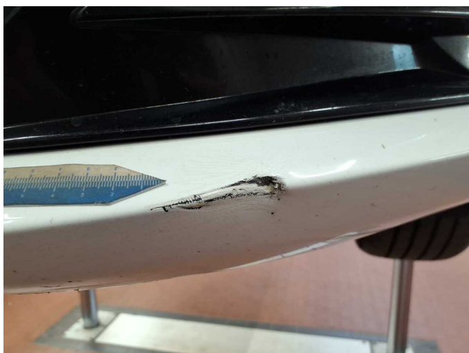
Damage 8: Front bumper: Front bumper - Deformed - Replace
