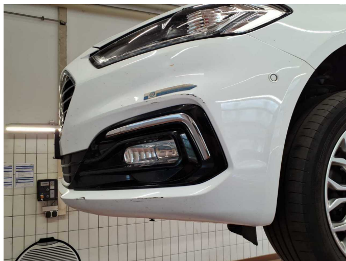
Damage 8: Front bumper: Front bumper - Deformed - Replace
