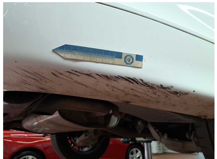
Damage 7: Rear bumper: Spoiler - Scratch(es) - Paint
