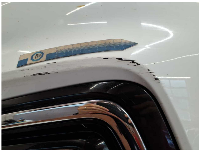
Damage 8: Front bumper: Front bumper - Deformed - Replace
