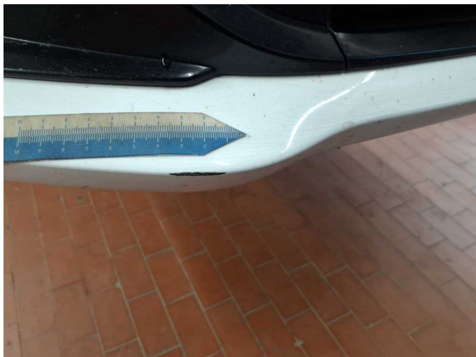
Damage 8: Front bumper: Front bumper - Deformed - Replace
