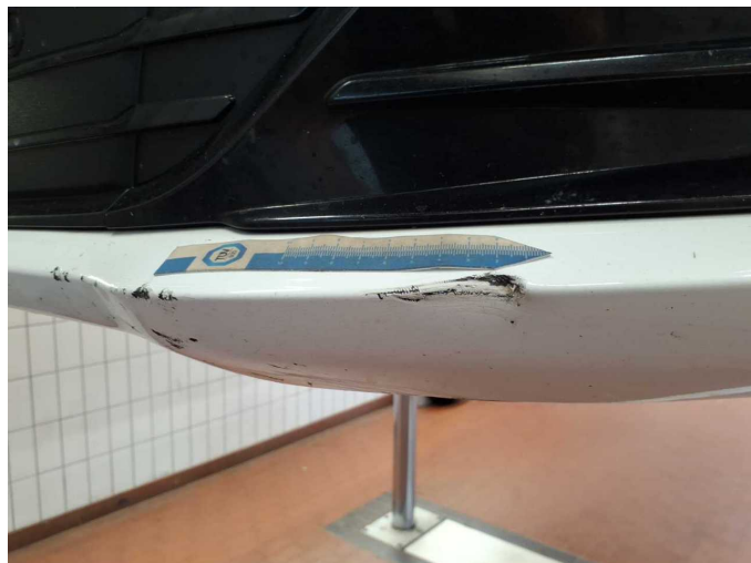
Damage 8: Front bumper: Front bumper - Deformed - Replace
