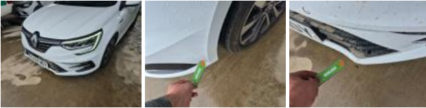
Bumper F, Scratch(es), Repair and paint (complete)
