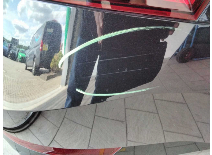
Damage 11: Rear bumper: Rear bumper - Scratch(es) - Paint
