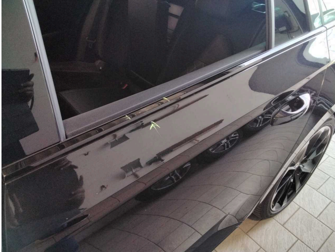
Damage 7: Door - rear left side: Strip - outer - Scratch(es) - Replace
