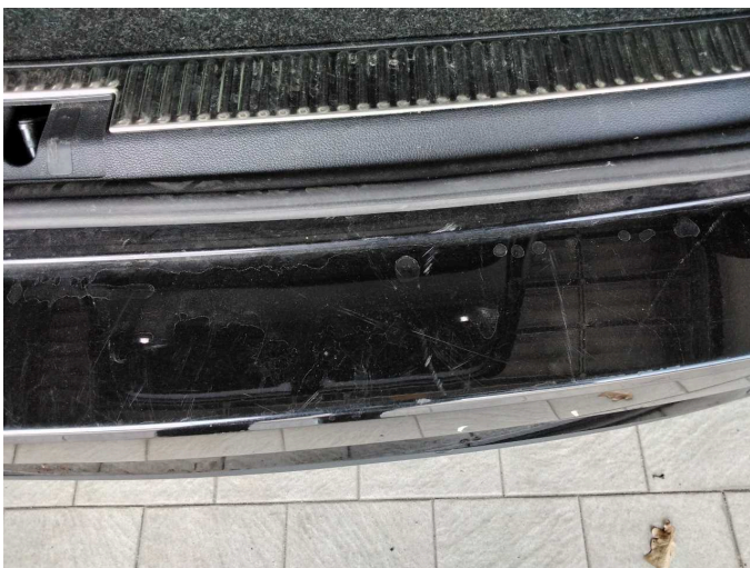
Damage 11: Rear bumper: Rear bumper - Scratch(es) - Paint
