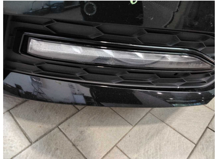
Damage 10: Fog lamp: Fog lamp - front right side - Leaking - Replace
