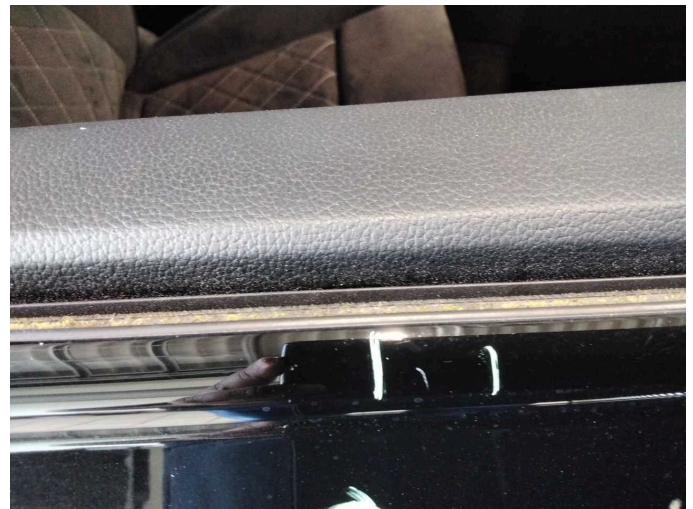
Damage 5: Door - front right side: Strip - outer - Scratch(es) - Replace
