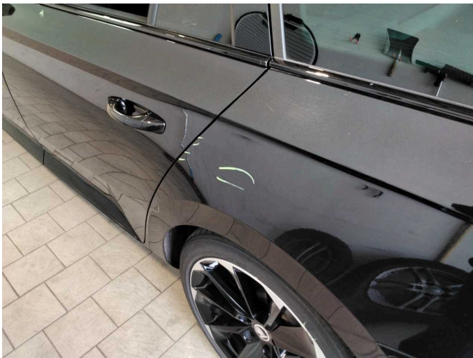
Damage 12: Side panel - rear left side: Side panel - Scratch(es) - Paint
