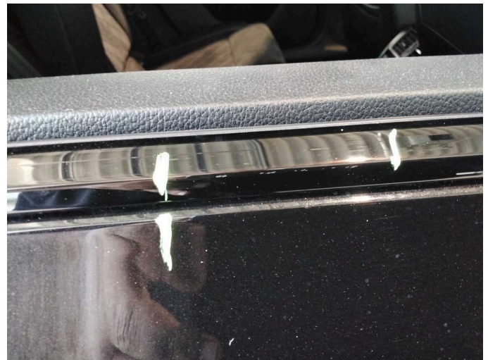
Damage 8: Door - rear right side: Strip - outer - Scratch(es) - Replace
