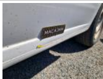
Side panel moulding L, Scratch(es), Replace
