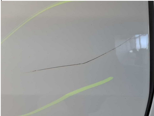
Damage #13: Door - rear right side: Door - Scratched - Repair and paint
