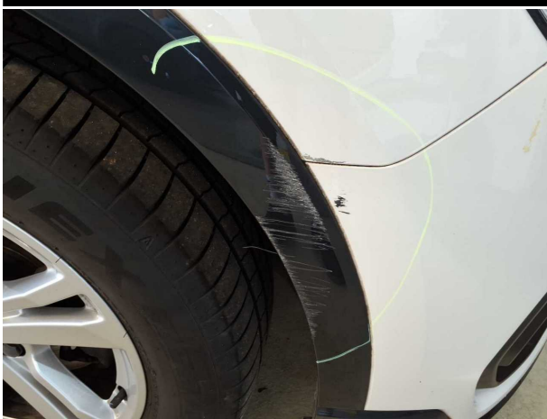
Damage #7: Mudguard - right side: Wheel well extension - Scratched - Replace
