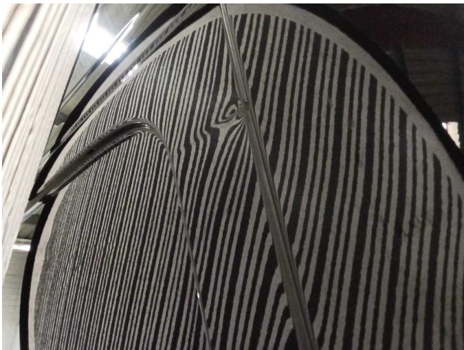
Damage 10: Side panel - rear left side: Side panel - Dent / paintcoat damage - repair according to calculation
