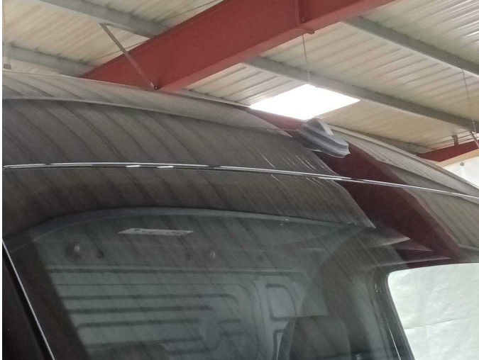
Missing part 1: Roof: Stub aerial - Missing - Perform
