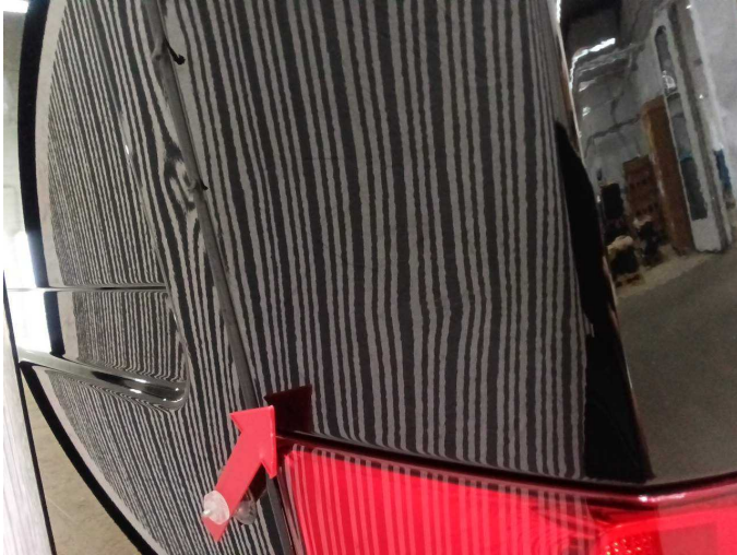
Damage 7: Body: D-pillar - left side - Dent / paintcoat damage - Smart repair
