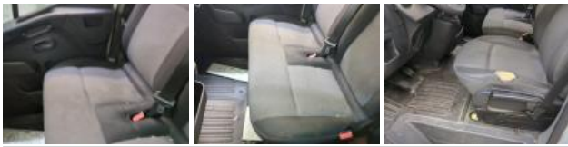
Seat cover FL, Worn, Replace
