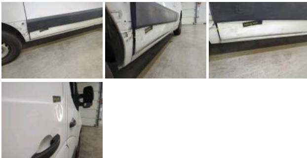
Door trim RR, Dent(s) and scratch(es), Replace
