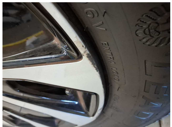
Damage 2: Wheel / tyres: Wheel cover - front right side - Scratched - Replace
