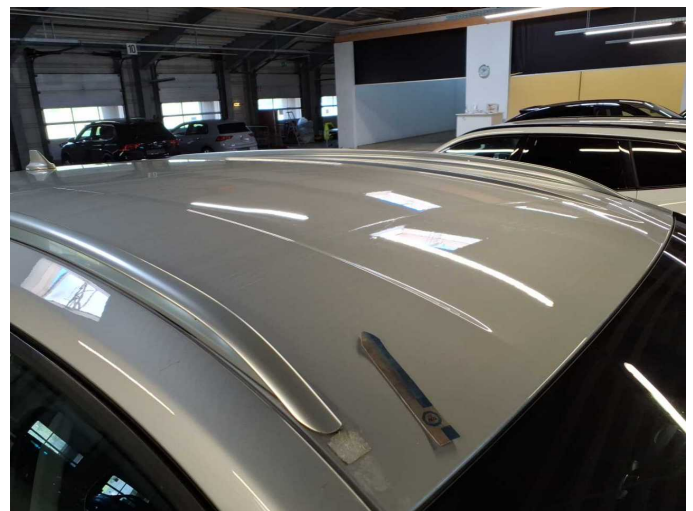
Damage 11: Roof: Roof - Scratch(es) - Paint
