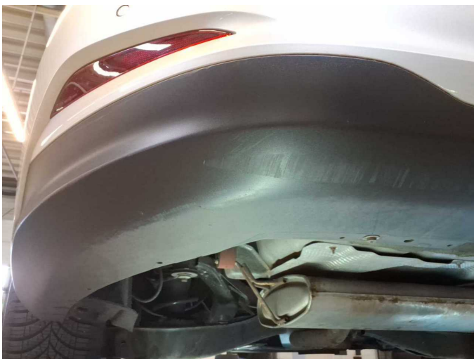
Damage 6: Rear bumper: Spoiler - Scratched - Replace
