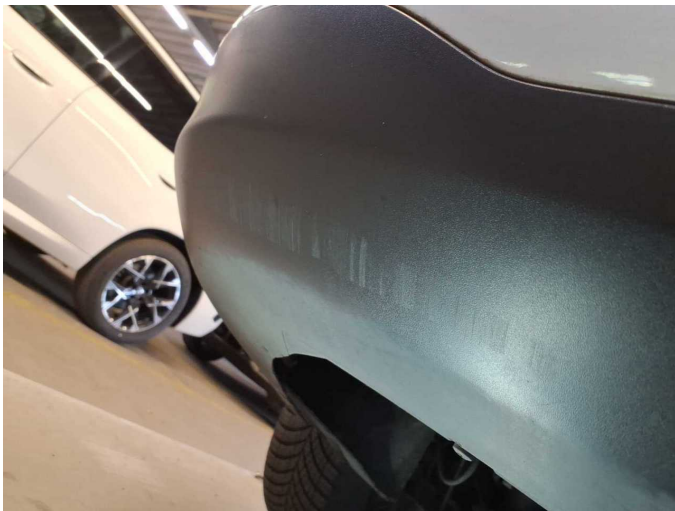
Damage 6: Rear bumper: Spoiler - Scratched - Replace
