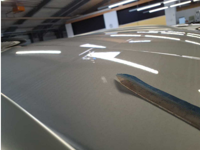
Damage 11: Roof: Roof - Scratch(es) - Paint
