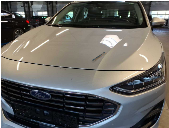
Damage 10: Bonnet: Bonnet - Deformed - Repair and paint
