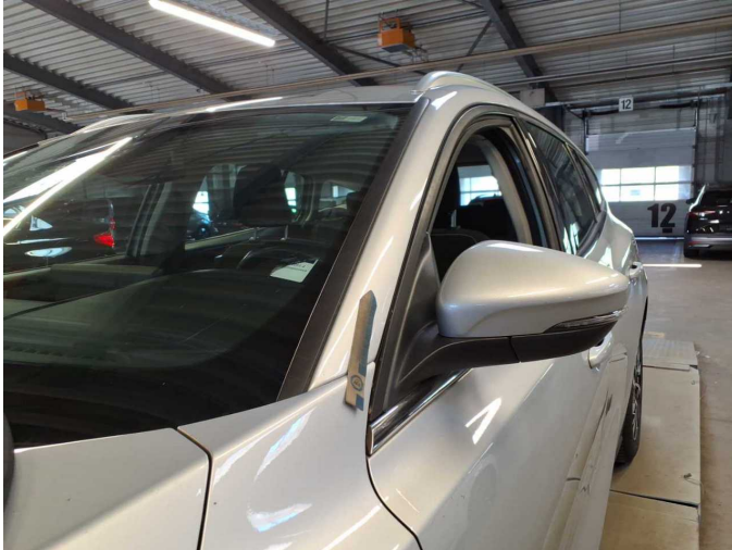
Damage 4: Body: A-pillar - left side (+Holm) - dent(s) - Smooth repair work
