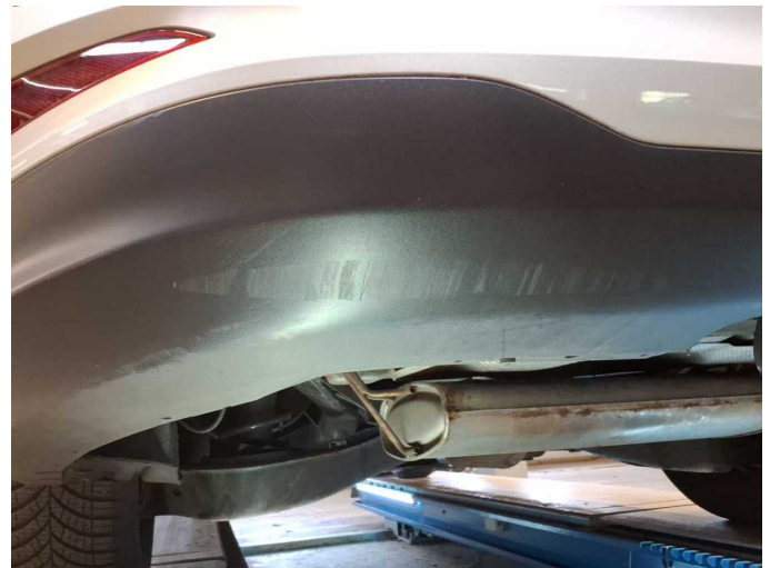
Damage 6: Rear bumper: Spoiler - Scratched - Replace
