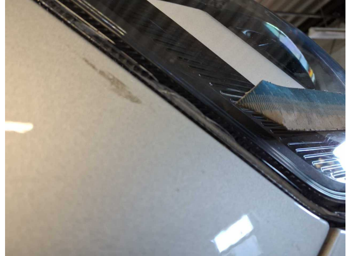
Damage 7: Headlight: Headlight - right side - Broken / torn - Replace
