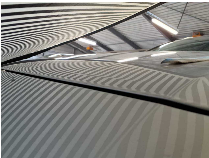
Damage 10: Bonnet: Bonnet - Deformed - Repair and paint
