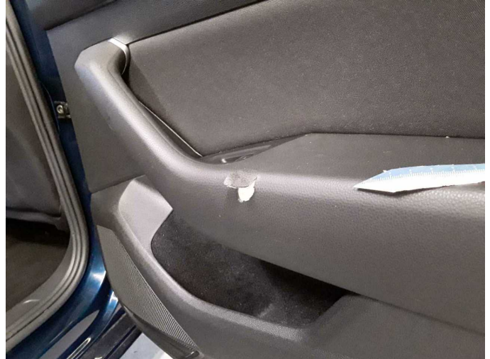
Damage 7: Trim / covers: Door trim - rear right side (Abdeckung Haltegriff) - Damaged - Replace
