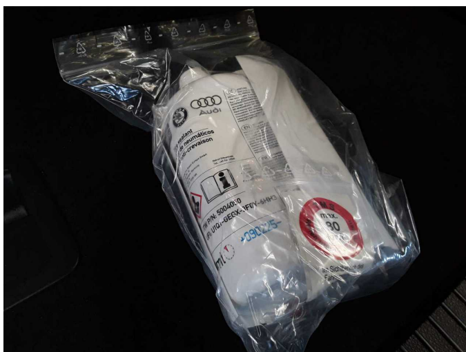
Damage 1: Equipment: Tirefit filler - Expired - Replace
