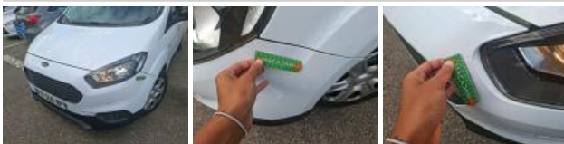
Bumper F, Bad repair, Repair and paint (complete)
