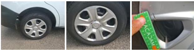
Tyre FR, Out of tolerance, Replace
