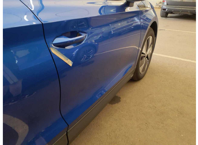
Damage 4: Door - front right side: Door edge - Scratch(es) - Smart repair
