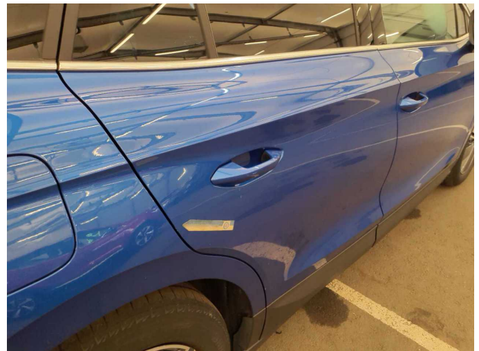
Damage 5: Door - rear right side: Door edge - Scratch(es) - Smart repair
