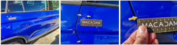
Door FR, Dent(s), Repair and paint (complete)
